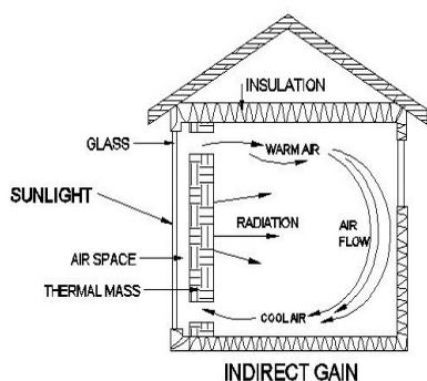
Fig. 2. Indirect passive solar energy. Thermal wall with ventilation for airflow
