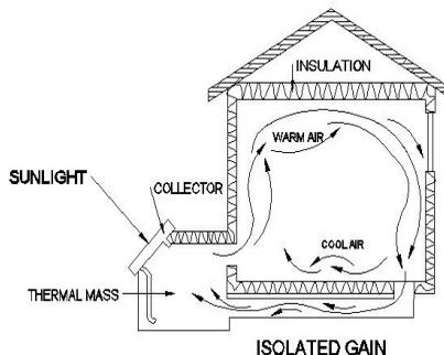
Fig. 3. Isolated gain passive solar energy.
