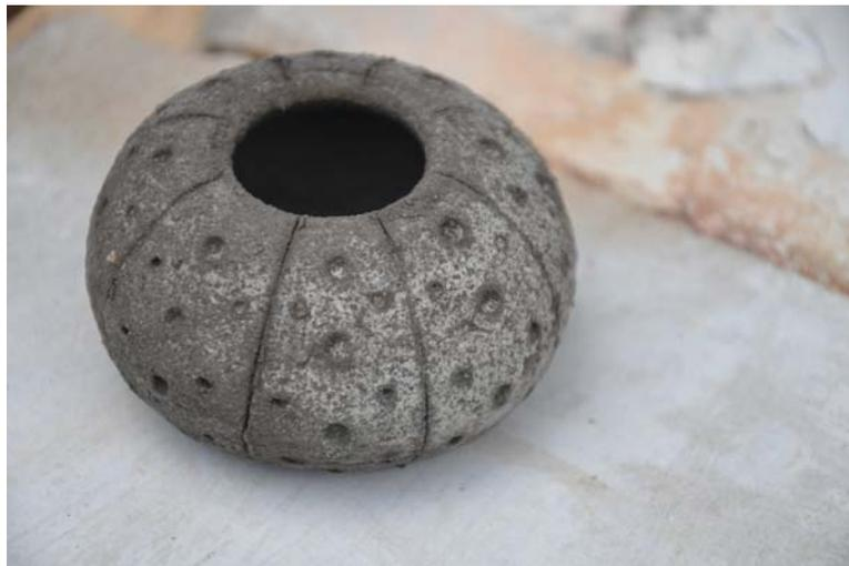
*Figure 6: Image of dry, collected clay showing evidence of salt precipitation on the surface*
