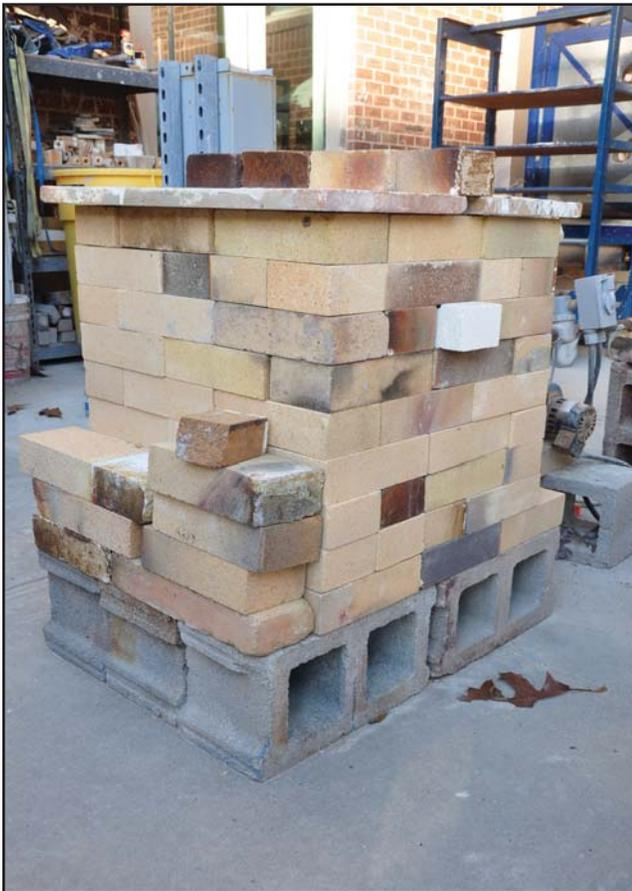
Figure 4: Image of small kiln built for firing the collected clay
