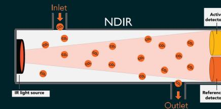
The K30 is a non-dispersive infrared (NDIR) sensor. It works by passing infrared light through a sample chamber and measuring the absorbance of that light, which is proportional to the concentration of CO<sub>2</sub> in the sample.
