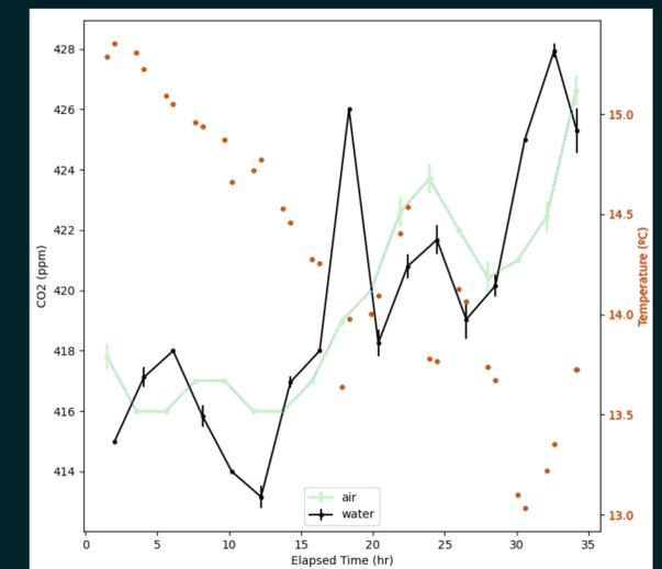
In a deployment off the floating dock at CMS, our team was able to obtain proof-of-concept data, as shown above. The average and standard deviation of the last 50 points of each sample is shown. ΔpCO<sub>2</sub> is the difference between lines.
