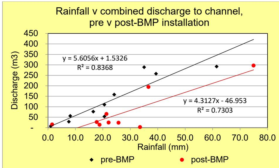
Figure 2: Total stormwater outflow (discharge) to Banks Channel in cubic meters as a function of rainfall (mm) for all 10 pre-BMP installation sampling events (black diamonds) compared to 10 post-BMP installation sampling events (red circles); from the north and south pipe combined.
