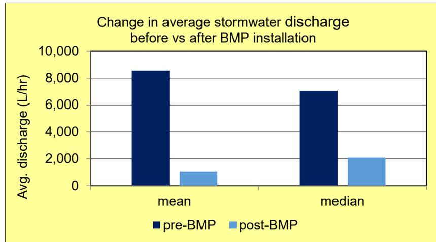
Figure 1. Change in average stormwater discharge (L/hr) to Banks Channel following BMP installation, north and south outfalls combined, comparison of 10 storms each.
