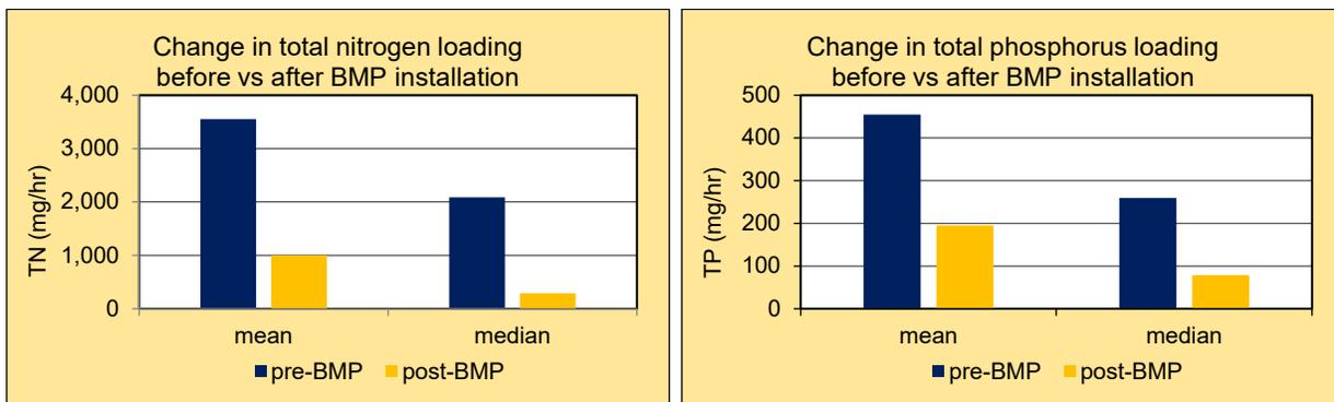
Figure 5 (left). Average total nitrogen discharge (mg/hr) to Banks Channel before vs after BMP installation, north and south outfalls combined. Figure 6 (right). Average total phosphorus discharge (mg/hr) to Bank’s Channel before vs after BMP installation, north and south outfalls combined.
