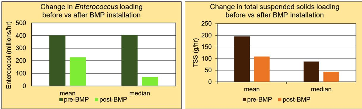
Figure 3 (left). Average *Enterococcus* discharge (millions of cell/hr) to Banks Channel before vs after BMP installation, north and south outfalls combined. Figure 4 (right). Average total suspended solids discharge (g/hr) to Bank’s Channel before vs after BMP installation, north and south outfalls combined.
