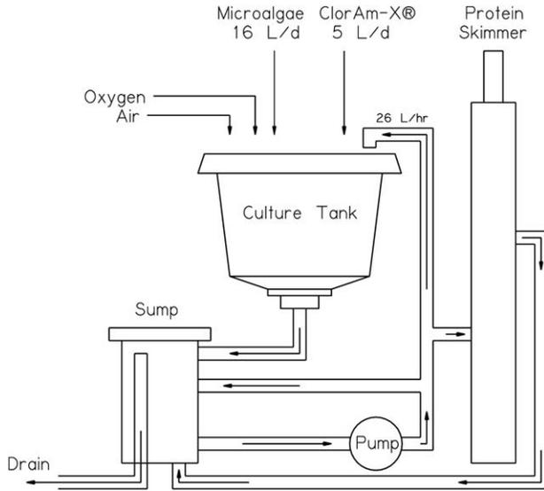
FIGURE 3. System schematic depicting pipe configuration and water flow.
