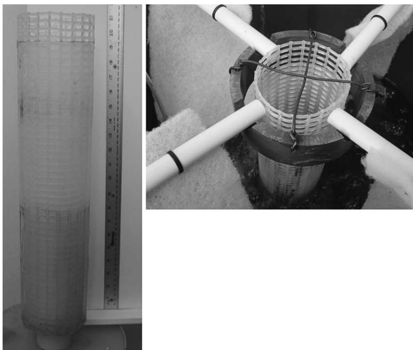
FIGURE 2. Center drain for culture unit with 55- $\mu\text{m}$  screen. Four filter mats are suspended from center drain.
